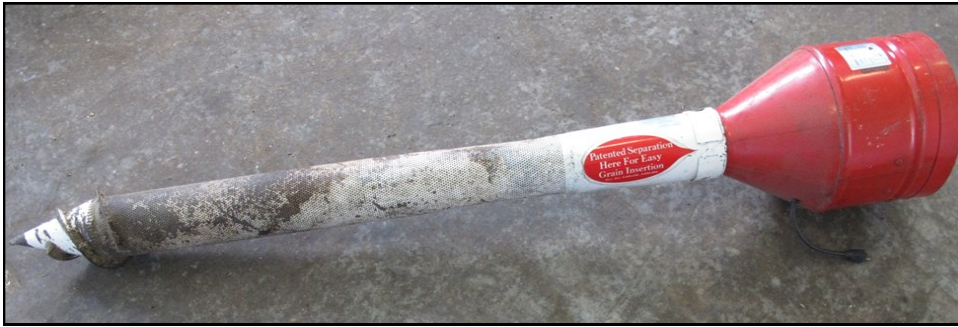
Figure 5-2. A screw-in auger is perfect for drying one-ton batches.
