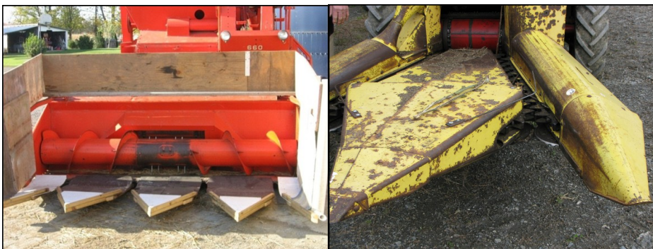
Figure 4-1. Left: homemade sunflower pans for a Case 660 combine (design by Roger Rainville, Borderview Research Farm); right: corn silage harvest head modified for harvesting sunflowers.
