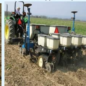
Zone-till planter follows ripped strips
