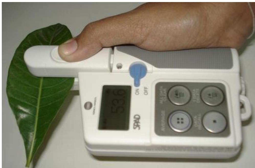
Figure 53. SPAD meter readings may be correlated with N status under certain conditions
