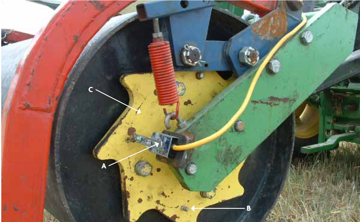
FIGURE 9.7. Side view of the smooth roller with crimping bar; (a) micro-switch, (b) engagement bolt with the switch's arm, and (c) eight-cam crimping bar control mechanism with clockwise rotation.
