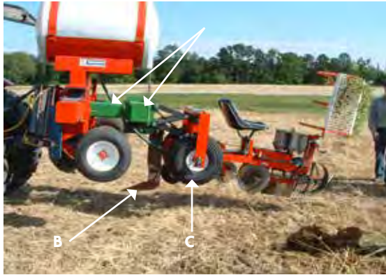
FIGURE 9.16. Side view of the modified RJ transplanter showing (a) the subframe with (b) the subsoiler shank and (c) two driving wheels to power the planting unit (left). Planting tomato seedlings into previously rolled/crimped rye using a modified RJ no-till transplanter from RJ Equipment Company (right).
