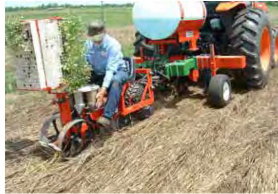
FIGURE 9.16. Side view of the modified RJ transplanter showing (a) the subframe with (b) the subsoiler shank and (c) two driving wheels to power the planting unit (left). Planting tomato seedlings into previously rolled/crimped rye using a modified RJ no-till transplanter from RJ Equipment Company (right).
