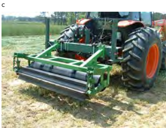
FIGURE 9.4. Roller/crimper for raised beds: (a) two rows and three furrows, and (b) one row and two furrows. A two-stage roller/crimper for smaller tractors (c).
