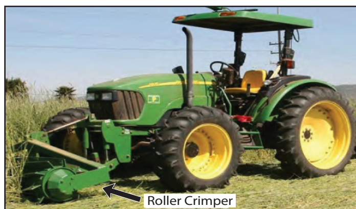
Figure 17: This rye cover crop was terminated using a roller crimper. (Eric Brennan)
