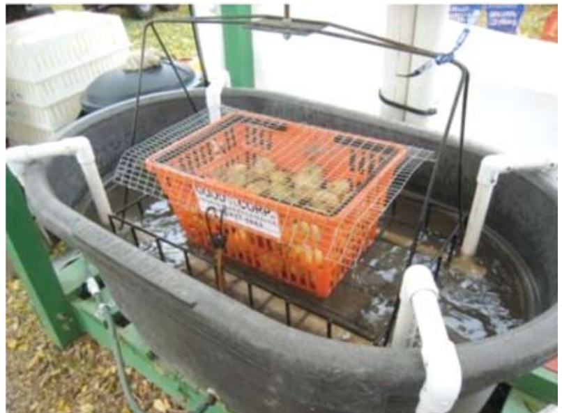
A motorized vegetable washer designed and built by Kevin Cooley saves water and washing time and frees up the person running the washer to do other tasks.
