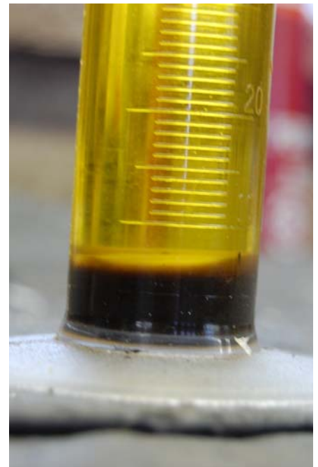
Fig. 2: 100 milliliters of canola oil collected at pressing time shows about 7 milliliters of sediment after 1 week of settling at room temperature.
