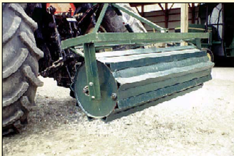
Figure 2. A homemade roller to kill cover crops (From USDA Farmer's Bulletin No. 2279).
