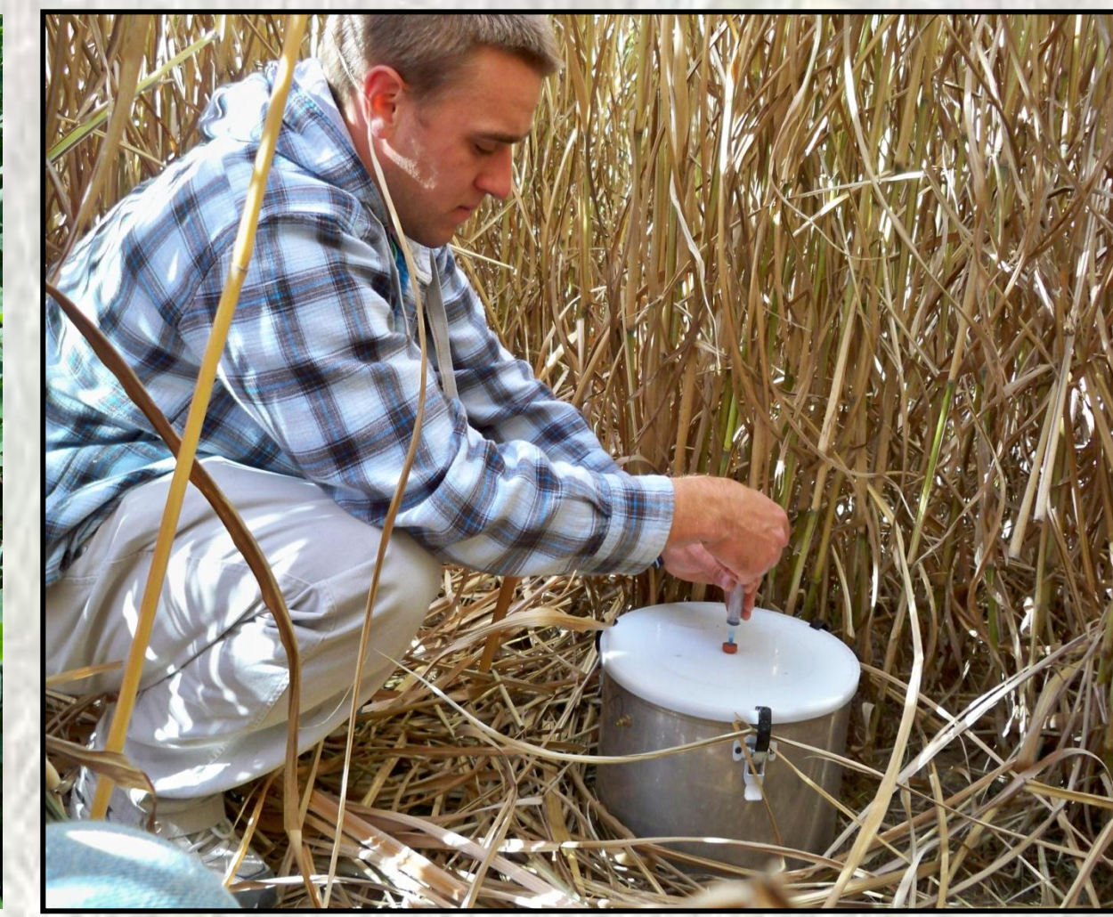
Figure 3. The cylindrical stainless steel chambers are designed for easy insertion, reflectivity, ease of sampling, and cost effectiveness. The vented chambers best resemble external environmental parameters and potential problems are minimized. The chambers are rugged and seal effectively.
