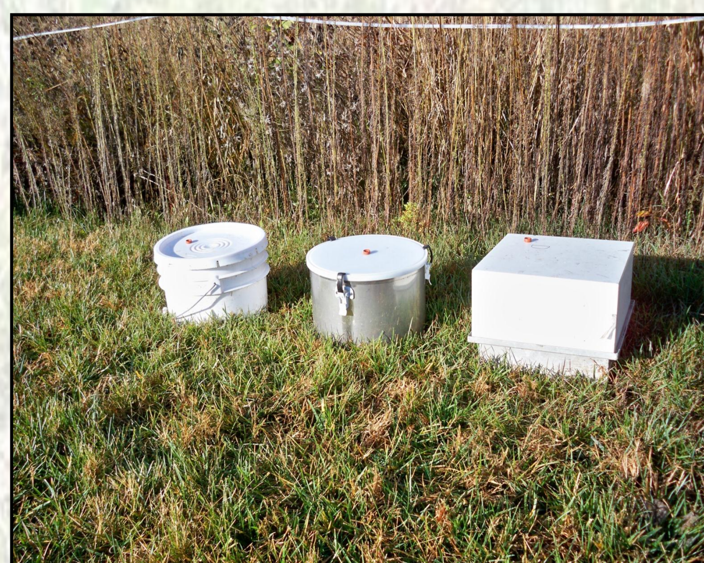
Figure 4 and 5. These images provide a side-by-side visual comparison of chambers during incubation (left) and open to the atmosphere (right). These chambers are similar in height, area/perimeter ratio, volume, and incubation duration. Technicians at KBS prefer the cylindrical stainless steel chambers because they are easy to deploy, the lid seal is more effective, and sampling is more efficient and practical. Currently, the LTER and GLBRC projects use hundreds of square and cylindrical stainless steel chambers.
