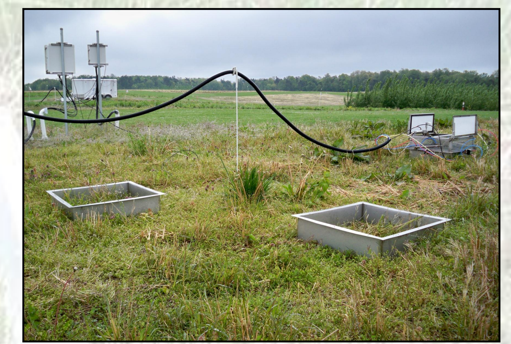
Figure 7 and 8. We also use automated chambers which provide a very good area/perimeter ratio. Coupled with an automated sampling system, these chambers provide the high flux resolution needed to capture short term events (rain, fertilization, tillage) that potentially drive GHG emissions in agricultural, grassland, and forest ecosystems. The automated chamber's expense and the technical expertise needed to operate limits its widespread deployment. Maximum temperature deviation from ambient during closure periods is 2C during warmer summer temperatures.
