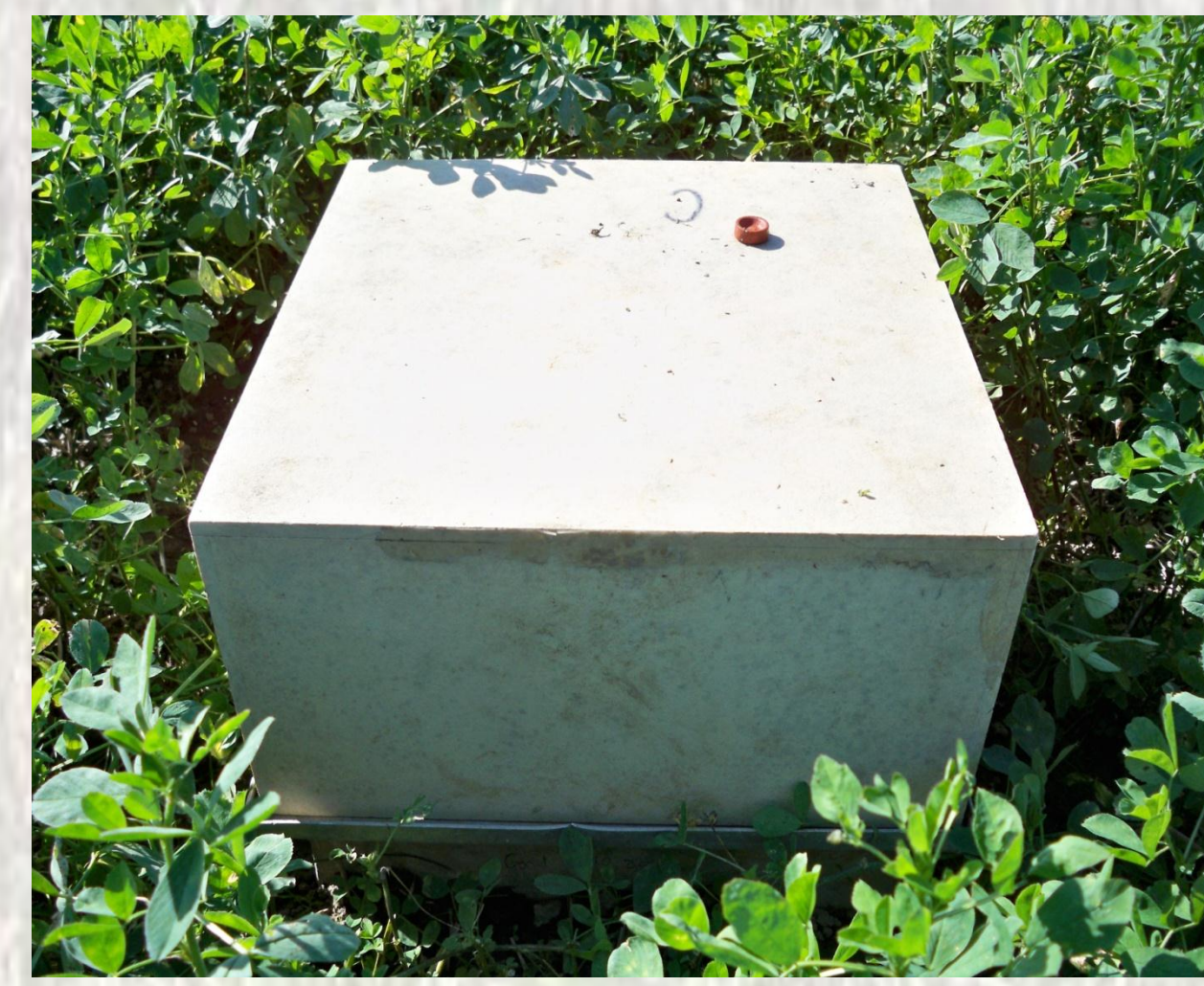
Figure 2. The square type chambers have a low vertical profile when installed with a base height of 5cm above the soil. These chambers are very expensive to produce and use a water trough around the base to create a seal. Technicians must use extra care to ensure that the water does not spill into the chamber prior to sampling. The square chamber has been seasonally deployed for over twenty years.
