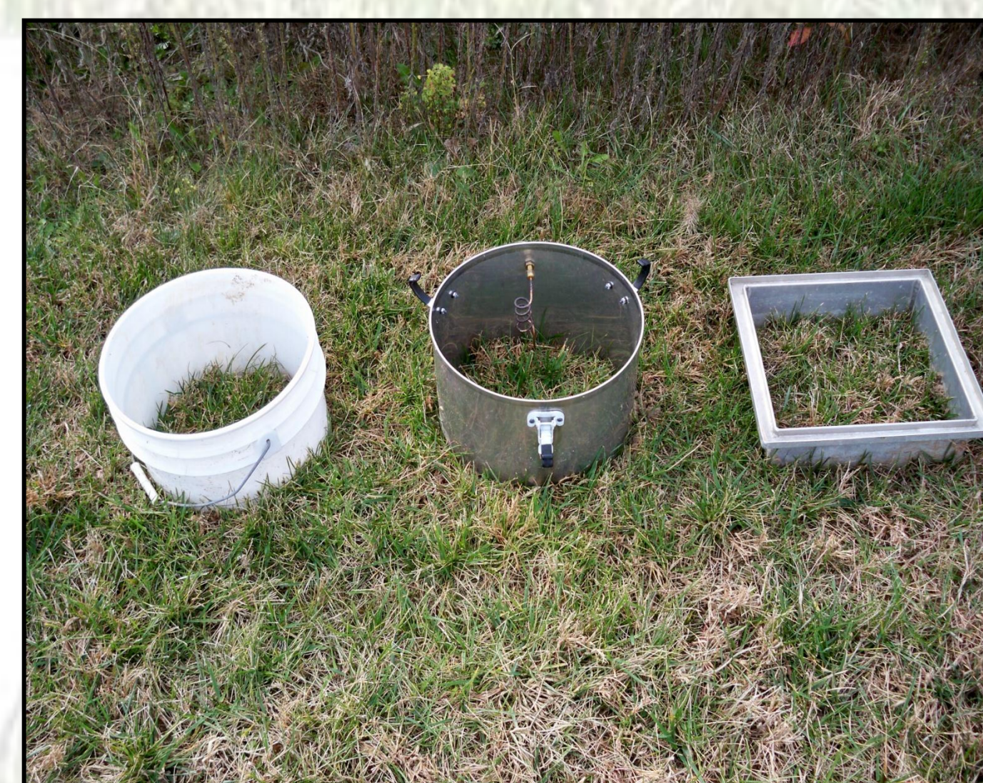
Figure 4 and 5. These images provide a side-by-side visual comparison of chambers during incubation (left) and open to the atmosphere (right). These chambers are similar in height, area/perimeter ratio, volume, and incubation duration. Technicians at KBS prefer the cylindrical stainless steel chambers because they are easy to deploy, the lid seal is more effective, and sampling is more efficient and practical. Currently, the LTER and GLBRC projects use hundreds of square and cylindrical stainless steel chambers.
