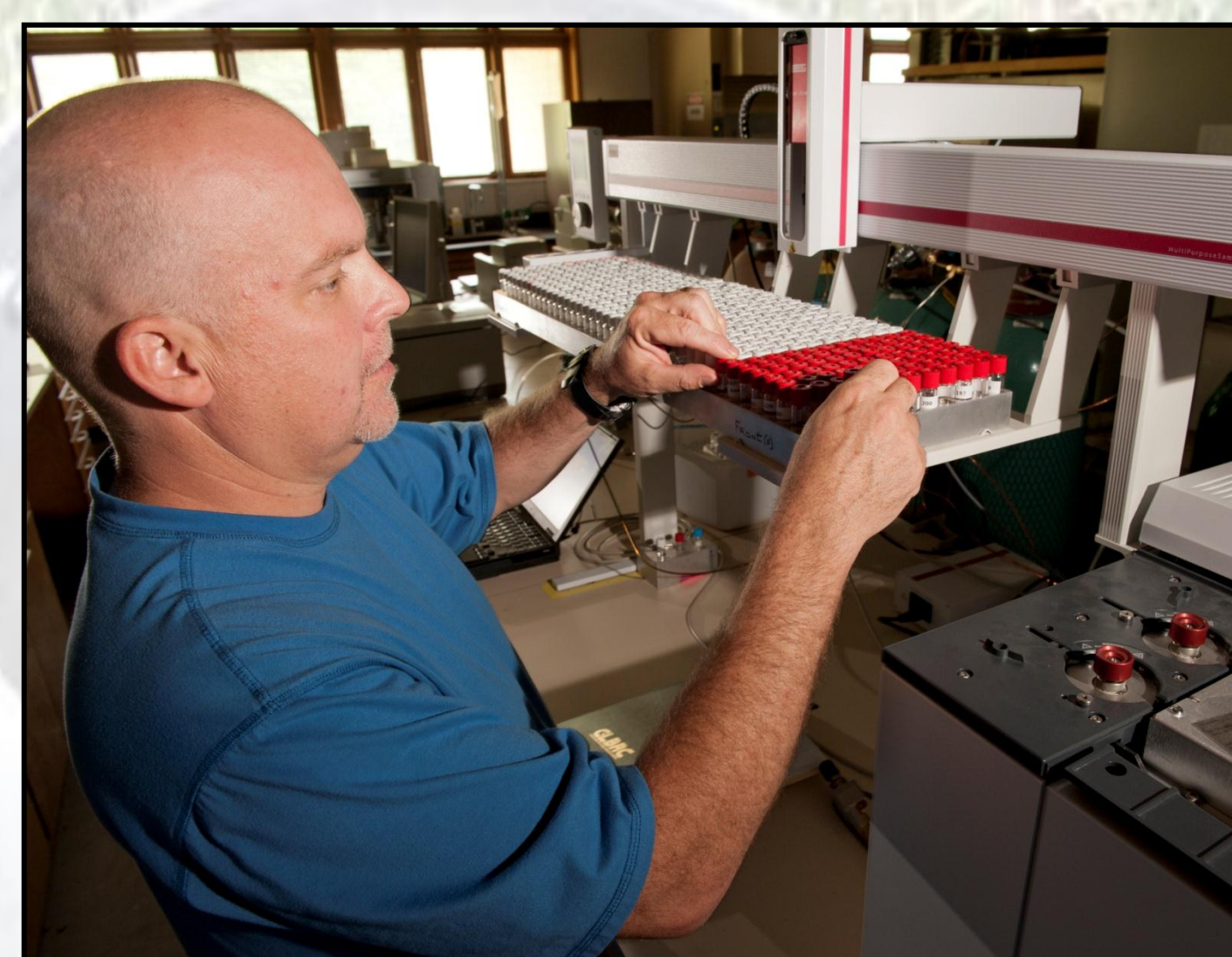
Figure 6. A Gerstel Autosampler is fitted to an Agilent GC for the analysis of N 2 O, CH 4 and CO 2 and is capable of sampling up to 440 vials per run. Currently, this system analyzes 40,000 samples annually. CV's for N 2 O, CH 4 and CO 2 at ambient concentrations are typically 1.0%, 1.5%, and 4% respectively.
