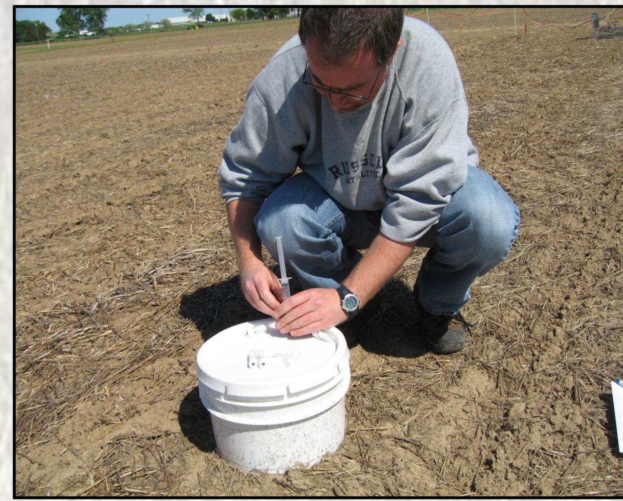
Figure 1. The bucket type static chambers are often used by individual researchers. KBS studies show more flux variability as the number of users/technicians per bucket chamber rises. A proper soil seal is more difficult to maintain and soil compression around the chamber is more frequent because of the force needed for lid removal. These chambers are very inexpensive.
