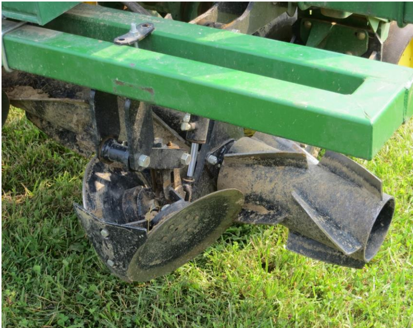
ZRX roller-crimper & row cleaner on parallel linkage Dawn Biologic ®
