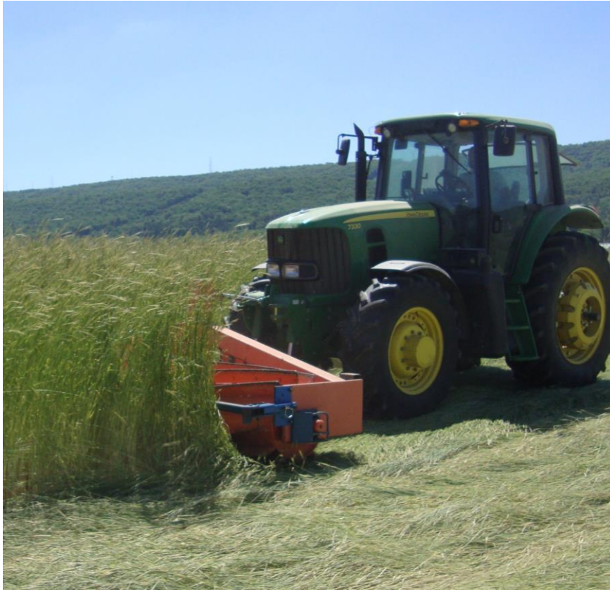
Cereal rye termination w/ roller crimper (3-4 tn/ac of dry matter)
